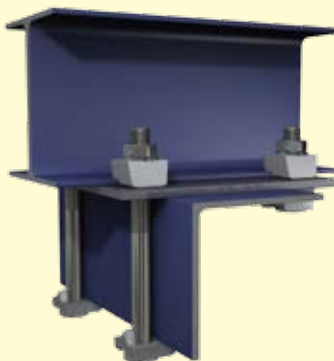
Angle section below an I-Section at 90 degrees
