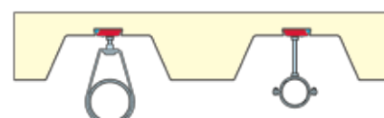
Typical pipe supports
