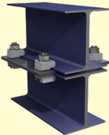
Two I-Sections of equal width running parallel
