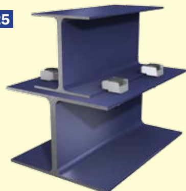
Drilled I-Section running parallel to another I-Section
