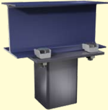
Column end plate to I-Section
