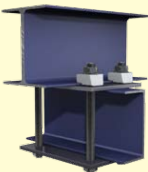
Channel section below I-Section at 90 degrees
