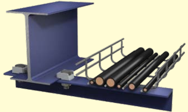
Cantilevered angle support for running cable tray
