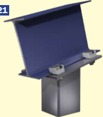
Column end plate to sloping I-Section
