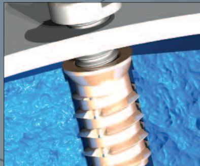
The Foamsert is a special version of the Trisert and has a very coarse truncated external thread form. Like the Trisert it has three equidistant cutting flutes over the length of the external form and it is this unique combination that makes the Foamsert ideally suited for use in structural foam materials, laminated chipboards, medium density fibre board and certain types of glass reinforced plastics.
