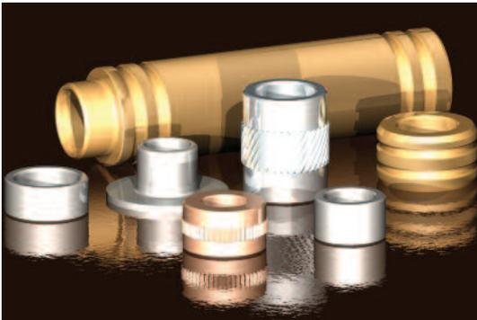
Anti-creep spacers are designed to provide reinforced clearance holes for bolts to pass through a plastic moulding, and thus allow metal-to-metal clamping forces to be applied to an assembly without over-stressing the plastic.
