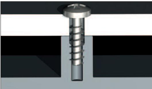
The Tappex TPX thread forming screws (not thread cutting) are designed to be used in most thermoplastic materials. These screws can be installed into drilled or moulded holes in a wide variety of applications.
