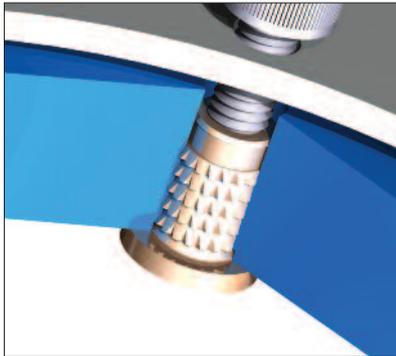
A barbed, double thickness headed insert available in short and regular lengths and two head diameter options. Available in a range of thread sizes from M1.6 to M10.
